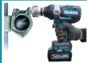
Auto-stop system available both in forward / reverse rotation modes
